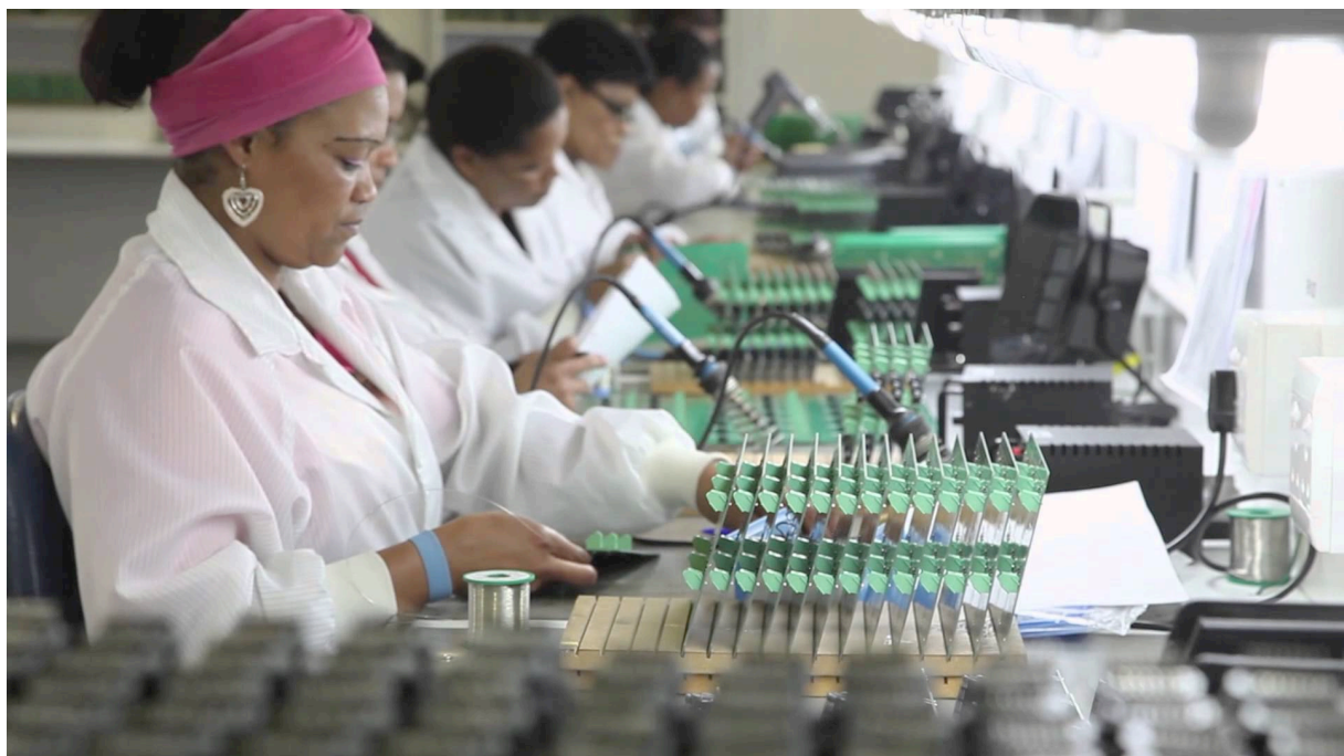
Figure 4.7: Manufacturing of the Nomanini devices (Nomanini website)
